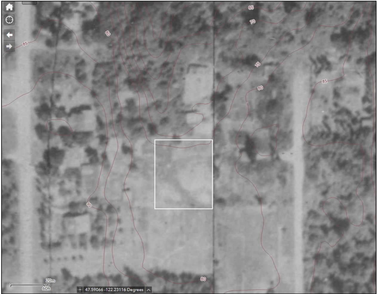
Figure 5. 1936 aerial photograph. Note absence of an open channel on the subject property (source: King County iMap)
